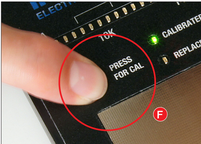
Press the CALIBRATION button once F
