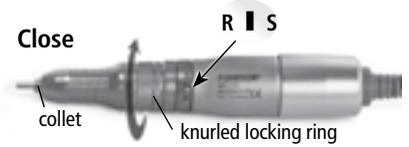
shanks less than 1" (25mm) long. To tighten the new bur twist the knurled locking ring counterclockwise toward the S (Secure) until it stops and locks the collet closed.
